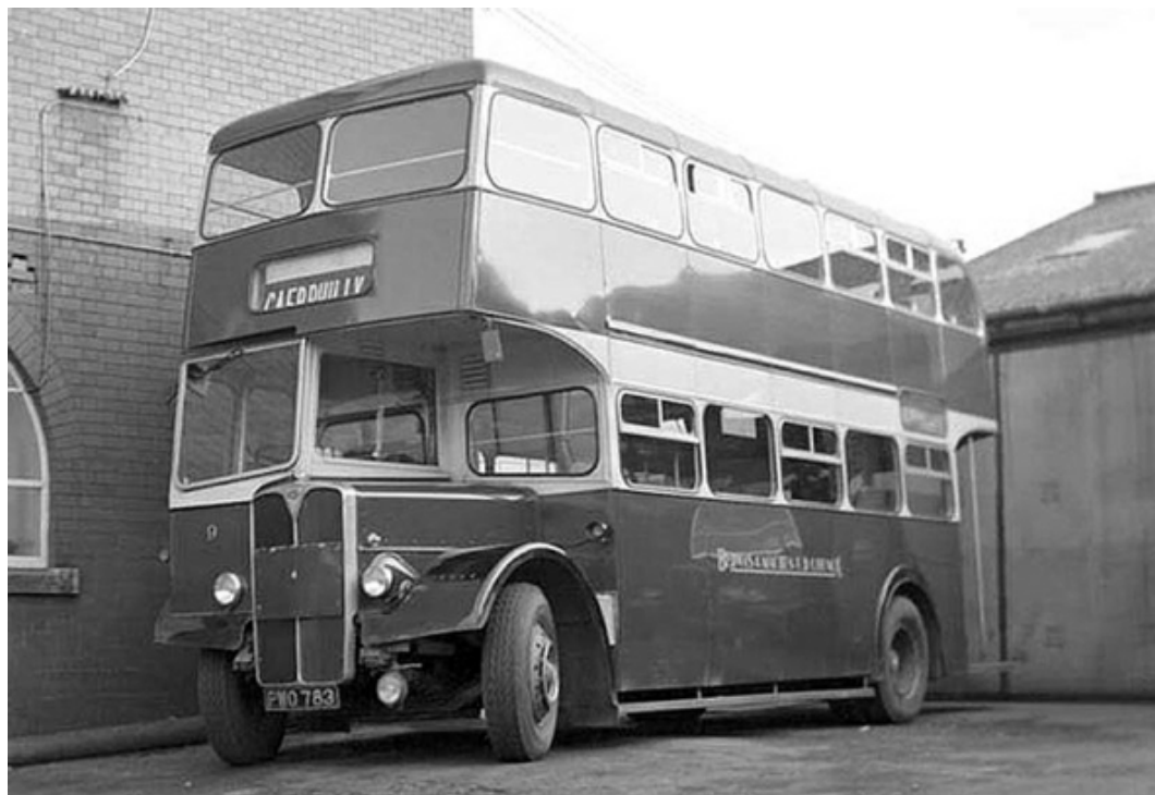
No. 9 (PW0783) a 1956 AEC Regent V looking more like a Regent III with its exposed radiator.
