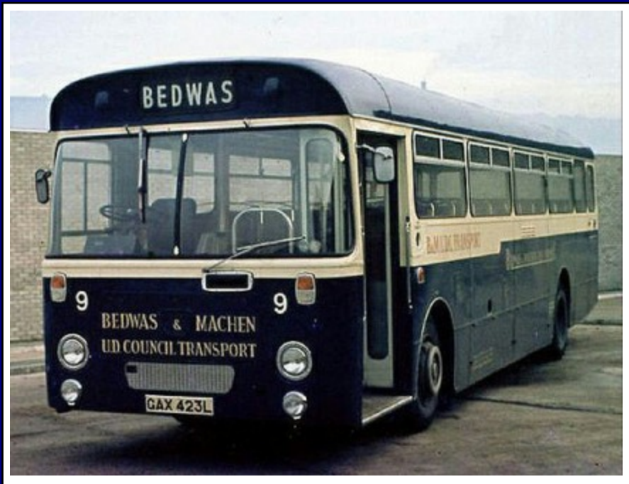
1972 Leyland PSU3B/2R No. 9 (GAX423L) with Willowbrook B53F bodywork. It became No. 93 in the Rhymney Valley District fleet in 1974.
